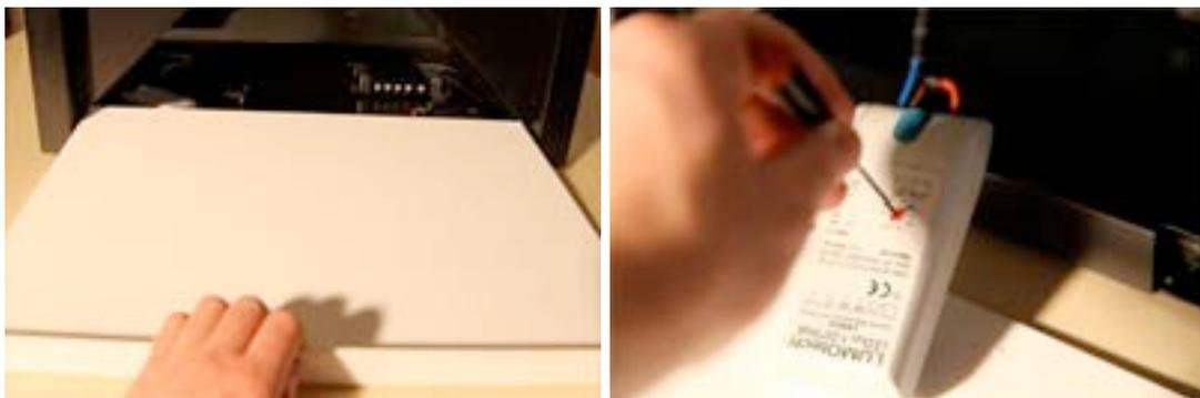
The Dreamoc also comes with a preinstalled light mask that focus the light in a smaller area inside the Dreamoc, and reduce the brightness of the lamp slightly. This light mask can be easily removed by pulling it down gently with a finger inside the mask.
